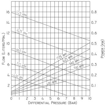
\* For pressures over 7 bar, the above selections are suitable for pumping fluids with lubricity (eq. oils, polymers). Service life will decrease for fluids without lubricity (eq. water, solvents).
