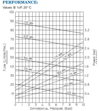
\* For pressures over 7 bar, the above selections are suitable for pumping fluids with lubricity (eq. oils, polymers). Service life will decrease for fluids without lubricity (eq. water, solvents).
